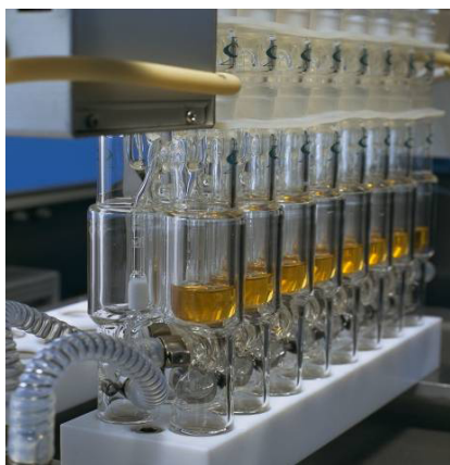
Picture 2 : Chemspeed's parallel reactor technology
