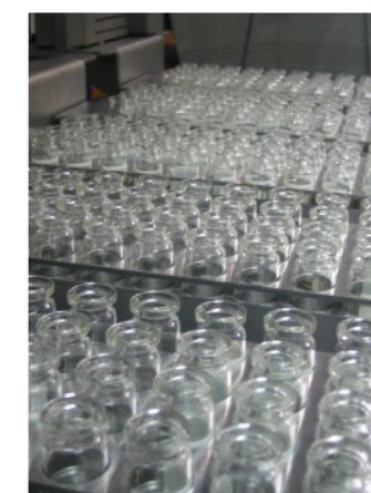
Tray view - 200 disposable automatically crimpable vials
