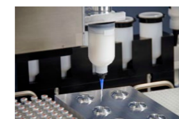
Overhead gravimetric dispensing of paste while mixing, heating and cooling (optional aspiration & heating for e.g. hot transfer)
