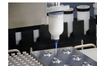
Overhead gravimetric dispensing of paste while mixing, heating and cooling (optional aspiration & heating for e.g. hot transfer)
