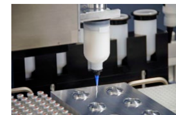
Overhead gravimetric dispensing of paste while mixing, heating and cooling
