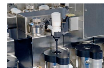
Overhead gravimetric dispensing of solid while mixing, heating and cooling in precision formulation vessel
