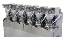
Process development workstation for 6 X 100 mL, 3 X 250 mL, 3 X 1'000 mL
