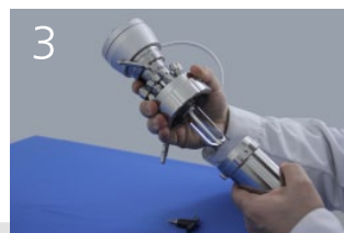
Plug in reactor
