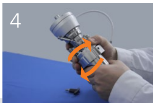
Screwless closing and self-sealing of reactor
