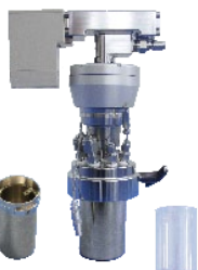
Materials of choice: glass, stainless steel (PEEK, PTFE or glass inserts available), Hastelloy, others on request
