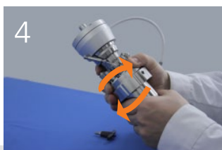
4 Screwless closing and self-sealing of reactor
