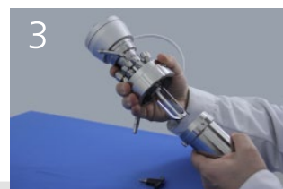
3 Plug in reactor
