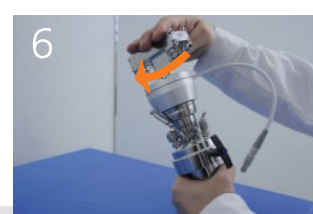
6 Screwless mounting and self-sealing of multiport drawer valve
