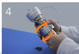
Screwless closing and self-sealing of reactor
