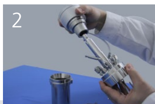
Mount cylindric magnetic stirrer drive
