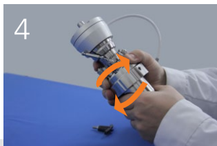
Screwless closing and self-sealing of reactor
