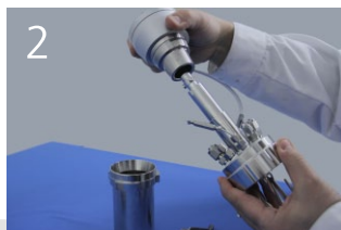
Mount cylindric magnetic stirrer drive
