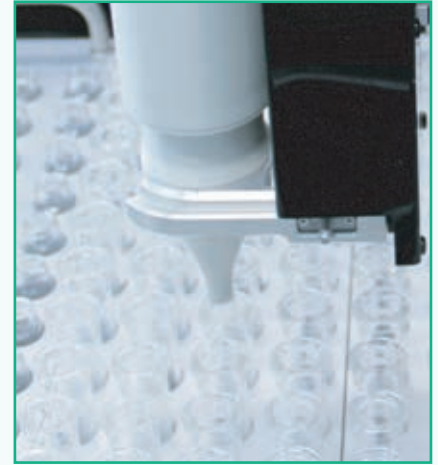
Gravimetric dispensing unit dispenses into destination while weighing
