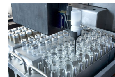
Gravimetric solid compound addition with overhead balance
