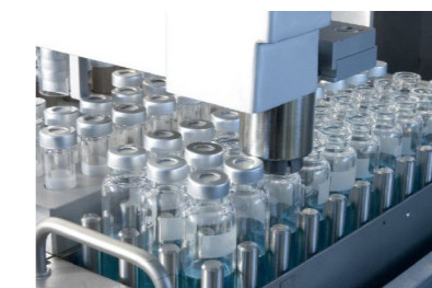
Vial capping and crimping
