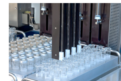
Gravimetric and volumetric liquid compound addition
